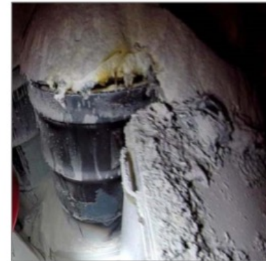
Figure 4-5. Analysis results for case with original estimate of properties and "slow" loading (left) matches observed damage seen in post-event photograph of Drum 68660 showing discoloration and lid displacement (right).
